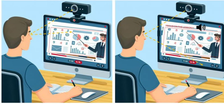
Figure 2: The first image shows eye gaze tracking as the user focuses on the AOI (red box). The second image displays a text prompt, "Focus on the screen," with audio feedback when the user's gaze shifts away from the AOI.
